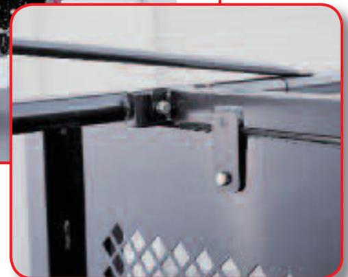
Platform racks are supported in front by the existing cab guard. The rear legs are height adjustable by cutting, with mount brackets that bolt to the platform body frame.
