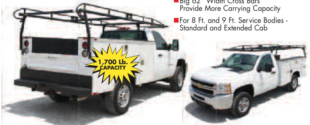
These highly crafted racks are quick to assemble and install. Rear leg mount brackets attach to the rear panel of the body. Brackets are located at the reinforced outside corner of the box where they can be raised or lowered without hitting tail lights. The height of the rack over the cab can be optimally set for all makes and models of truck or service body. Mount brackets set the legs off 5/8" from the rear panel to accommodate top opening boxes.
